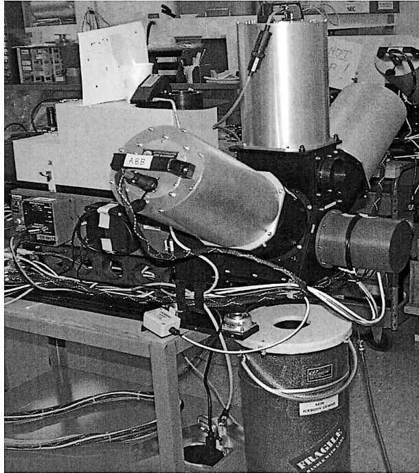
FIG. 5. Typical UW-SSEC laboratory end-to-end calibration verification using reference targets at about 318 (zenith view) and 273.15 K (nadir view). This “four body” test was used to verify the radiometric calibration of the AERI instruments prior to deployment of the systems to the DOE ARM sites.
