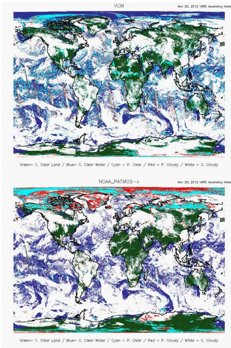
Figure 1. Results from the VCM (top) and PATMOS-x (bottom) cloud mask algorithms applied to VIIRS for data collected in ascending orbit on November 29, 2012.
