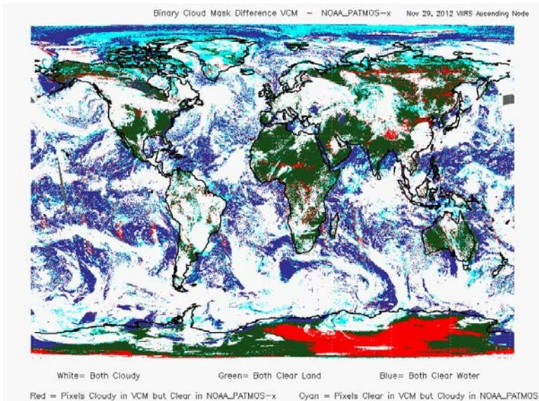
Figure 2. Differences between the VCM (top) and PATMOS-x (bottom) cloud mask algorithms applied to VIIRS for data collected in ascending orbit on November 29, 2012. Green and blue regions are where both methods detect clear over land and water, respectively. Regions colored cyan indicate where the VCM detected clear while the PATMOS-x detected cloud; red pixels are where the VCM assigned cloudy and PATMOS-x clear.
