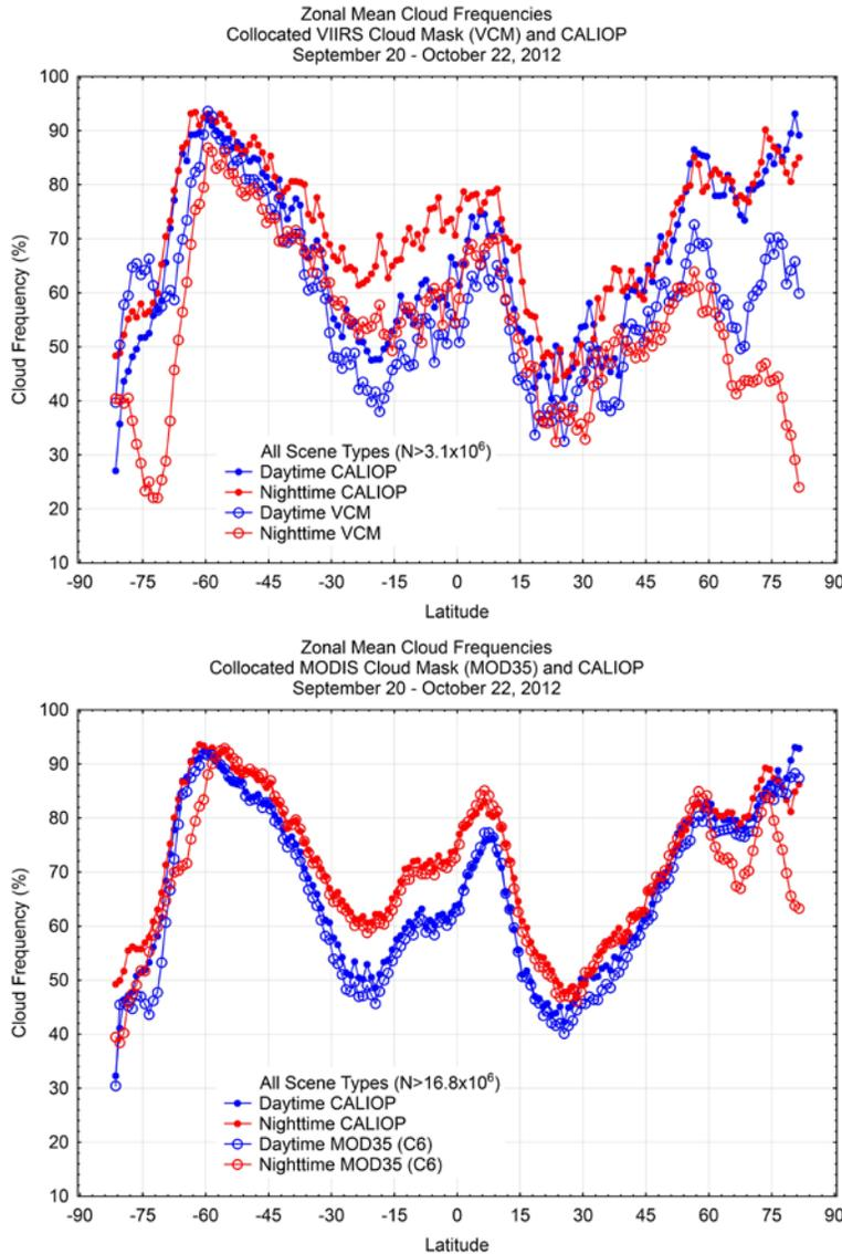
Figure 3 Zonal mean cloud frequency for CALIOP and VCM (top) for the period September 20 through October 22, 2012. The bottom figure shows the same comparison for CALIOP and MODIS MOD35 Collection 6 algorithm.
